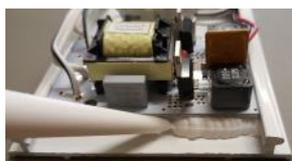
Put the sealant between the inverter and the base.
