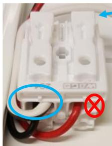
First the 'ground' cable (white) has to be inserted into the existing connector as shown in the picture above
