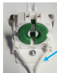
Put the lamp holders (2 x) (which are already connected to the new inverter) back into the brackets
